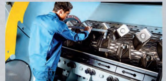
The Lindner modular system enables you to choose between different forms of motorization, cutting systems and screens – and you can optimize the machine specifically for your applications.
