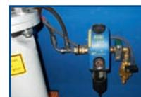
Water sprinkler system for dust collection
